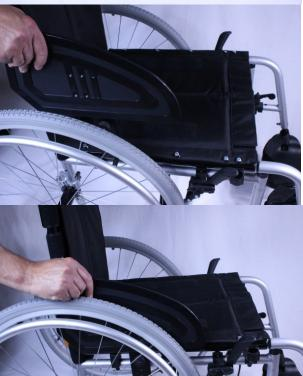
After adjusting the height and length of the side guard, insert the side guard band in the side guard mounting socket.
