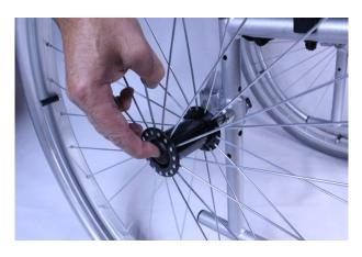
The wheelchair is equipped with quick release axles.
