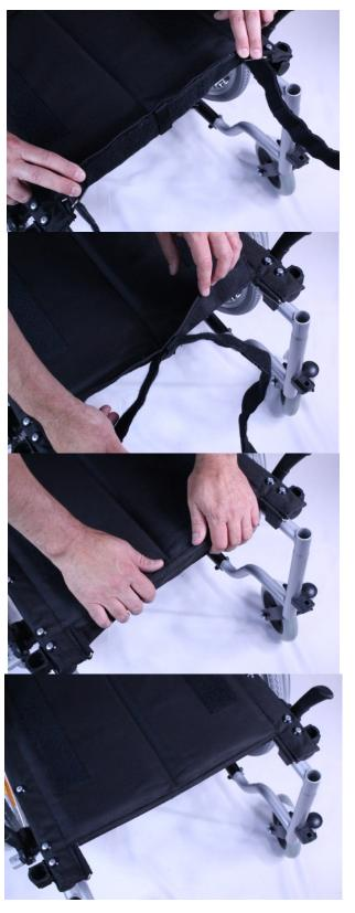
To reduce the seat depth, undo the Velcro strap under the seat.
