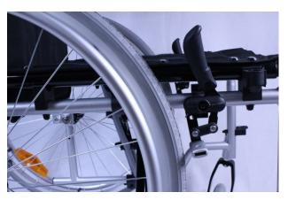
The brake can be adjusted according to the rear wheel position and tyre type/ dimensions. Slide the brake along the frame tube to the desired position.
