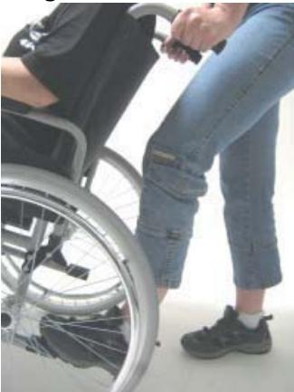
Push the bottom rail rear end down while pushing down and back on the push handles.
