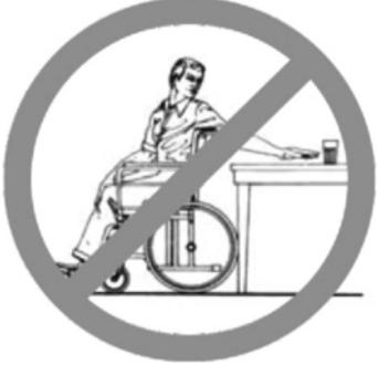
Propel the wheelchair as close as possible. When stretching and bending, do always have full contact between the backrest and the back otherwise the wheelchair may tip over. Stretching behind the back is not recommended.
